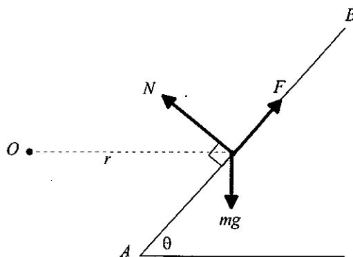
The diagram shows the forces exerted on a car of mass  $m$  travelling at speed  $v$  on a banked circular track  $AB$  of radius  $r$ . The track is banked inwards at  $\theta$  to the horizontal. The road exerts the normal force  $N$  at right angles to the road and there is a frictional force  $F$  exerted up the track.
